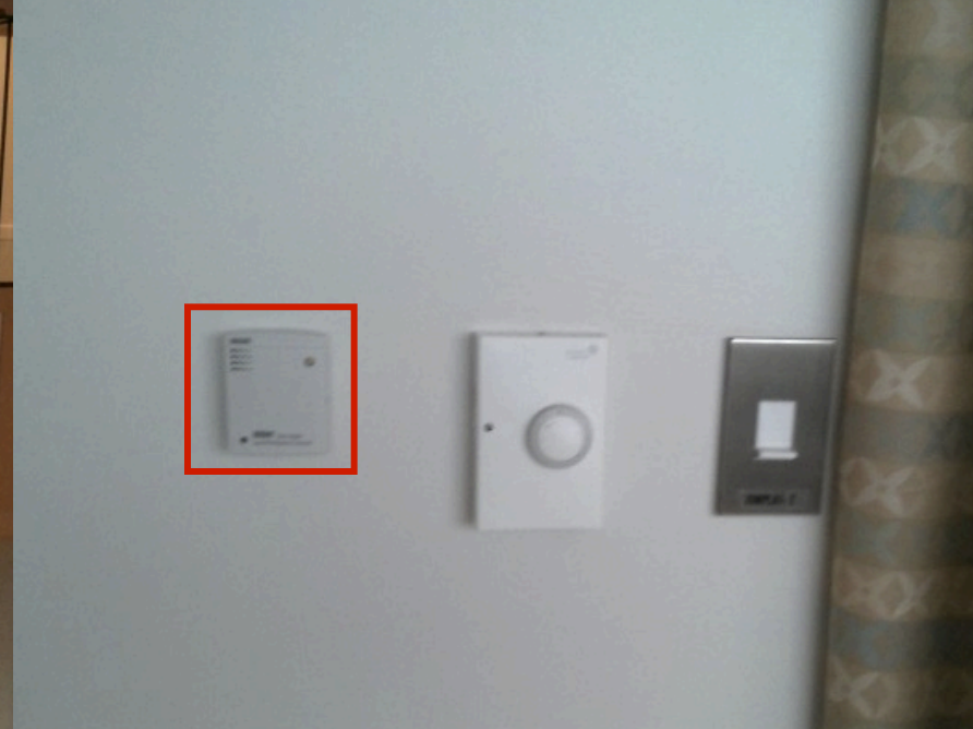
Data Logger (attached with adhesive) measuring temperature, relative humidity and light
