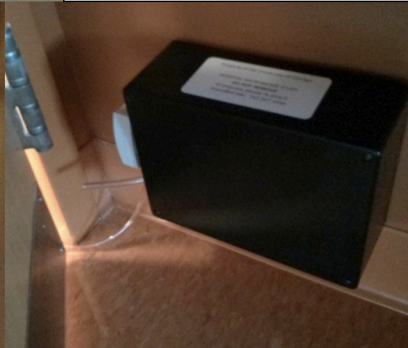
Differential Pressure Sensors (in black box with batteries, attached with adhesive), data logger, clear tube running to outer door frame
