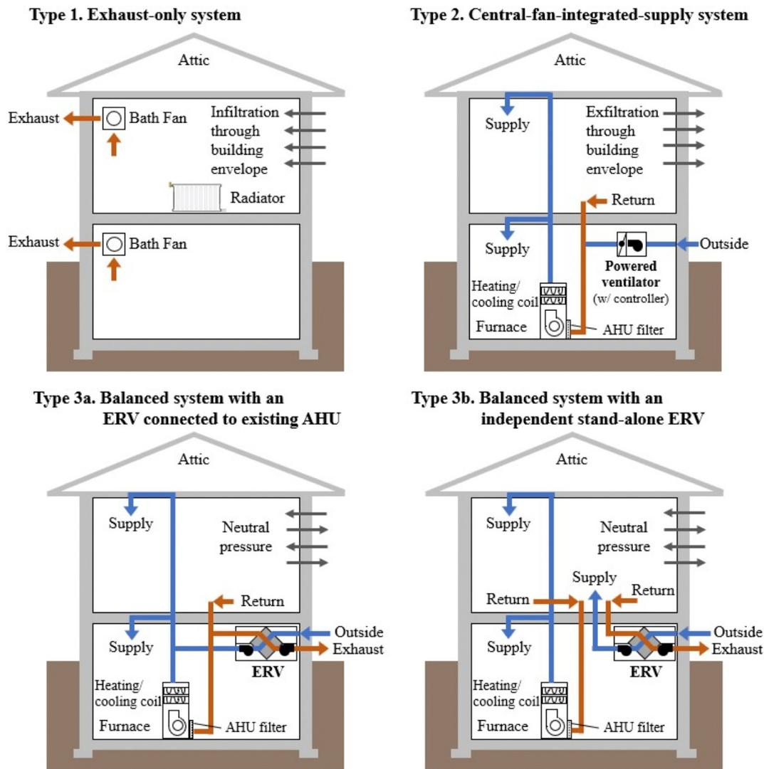
Fig. 3. Diagrams of the three main types of mechanical ventilation systems installed in the study homes.
