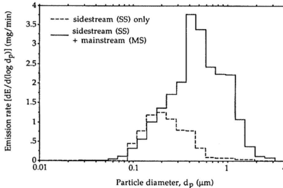
**FIGURE 1.** Effective particle emission rate from a burning cigarette as a function of particle diameter. The form of the figure is such that the area under a curve between two particle sizes is proportional to the mass emission rate of all particles within those size limits. These experiments were reported by Sextro et al. (1991). The emission profiles are based on a presumed particle density of  $1.4 \text{ g cm}^{-3}$ .
