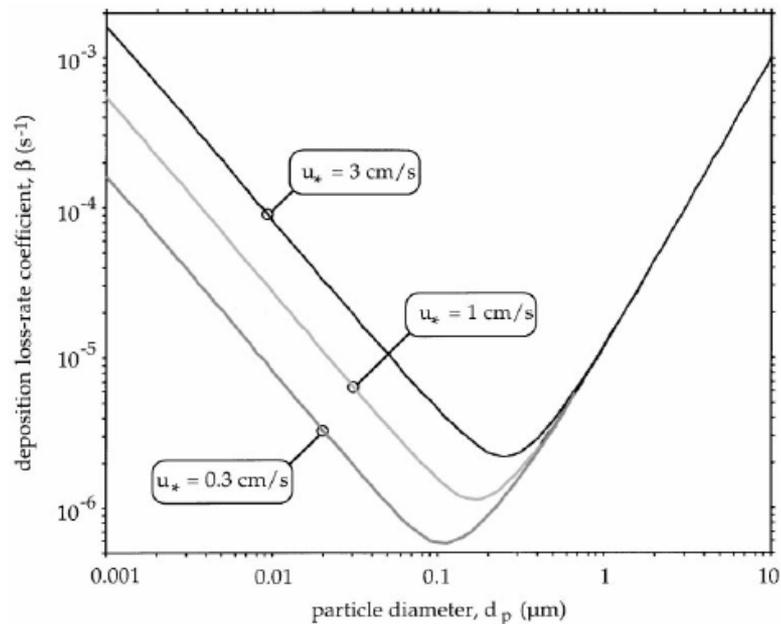
Fig. 5. Particle deposition loss-rate coefficient,  $\beta$ , for typical room dimensions (3 m high  $\times$  4 m  $\times$  5 m) according to the current model. Friction velocities of 0.3–3  $\text{cm s}^{-1}$  approximately span the range expected for mechanically ventilated indoor spaces. Predictions assume air pressure is 1 atm, temperature is 293 K and particle density is  $1.0 \text{ g cm}^{-3}$ .
