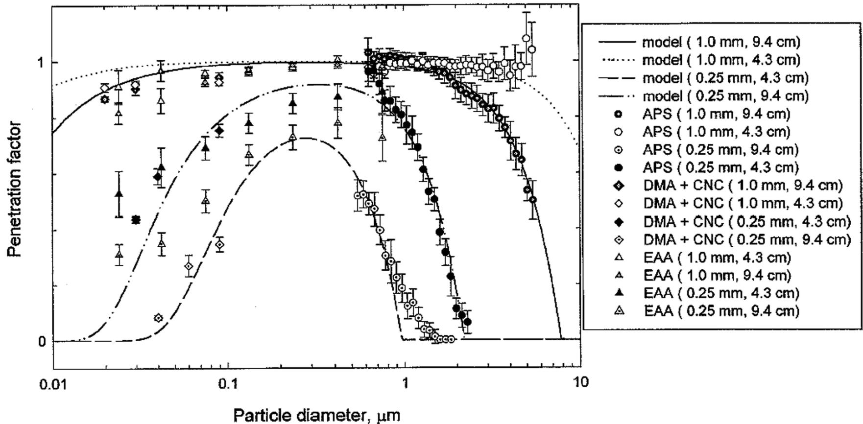
**Figure 5.** Comparison of model predictions with experimental data for aluminum cracks. Results are presented for four sets of crack dimensions (crack heights of 0.25 mm and 1.0 mm and crack flow lengths of 4.3 cm and 9.4 cm), with an applied pressure difference,  $\Delta P = 4$  Pa.
