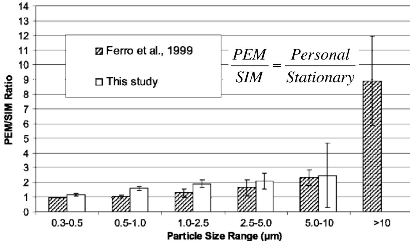
**Figure 4.** PEM/SIM ratio by particle size during human activity periods for two independent studies. Ferro et al. (1999) collected personal and indoor concentrations using Met-One Model 237B laser particle counters for six vacuuming experiments in a separate Redwood City, CA, USA, residence.
