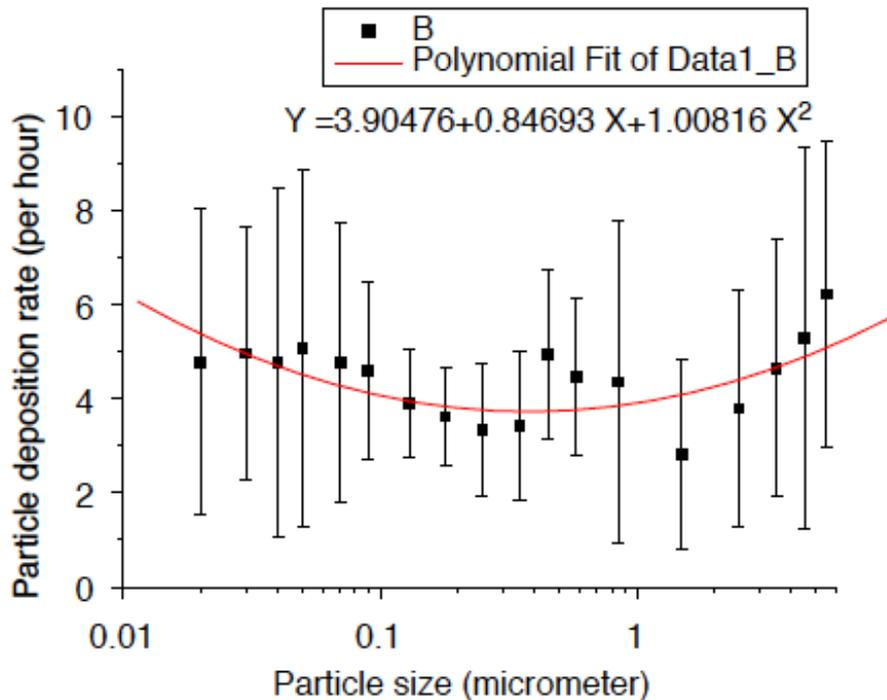
Fig. 3. The average of particle deposition rates for the 18 particle size intervals under normal ventilation conditions (Error bars represent one standard deviation). The polynomial fit line with the correlation coefficient ( $R^2 = 0.33$ ).
