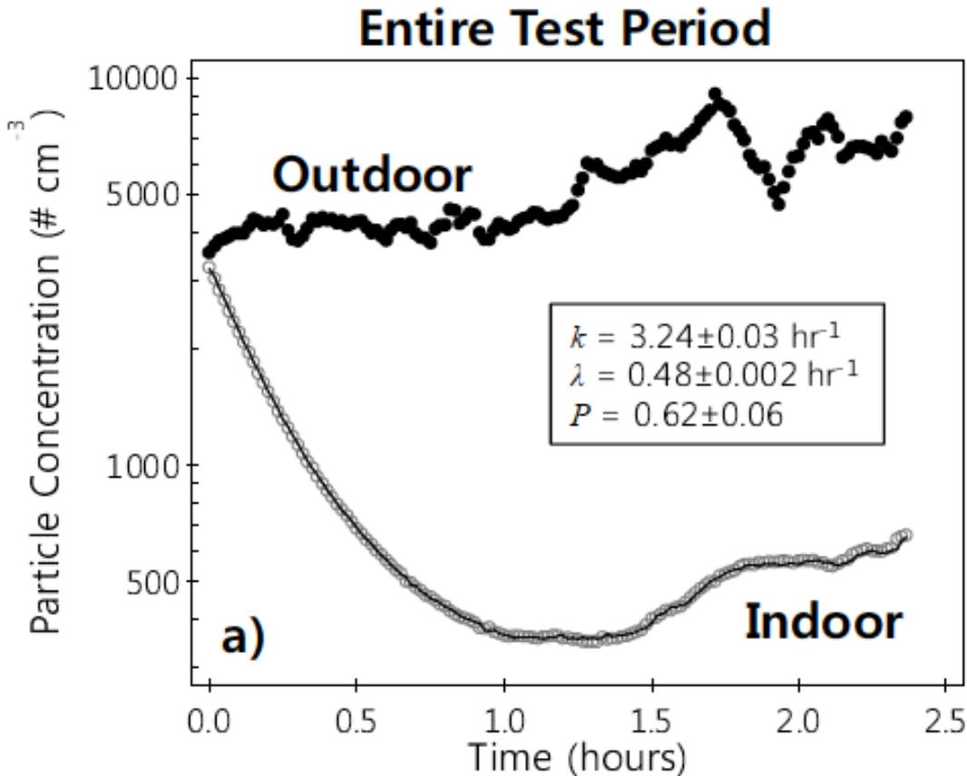
$$C_{in,t} = C_{in,t-1} + (P\lambda C_{out,t-1} - (\lambda + k)C_{in,t-1})\Delta t$$
