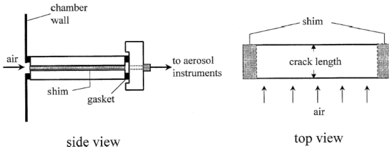
**Figure 1.** Configuration of crack apparatus (not to scale).
