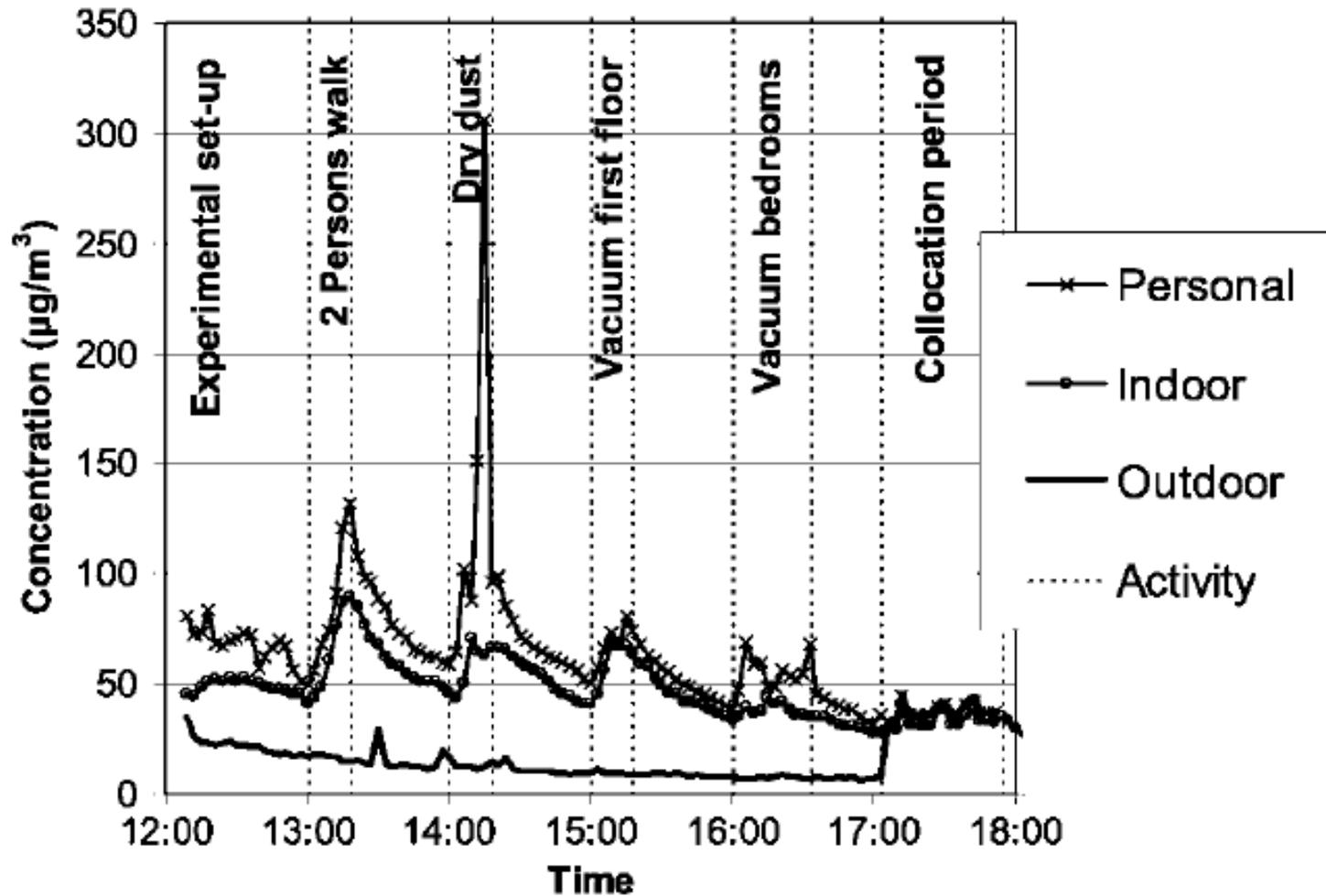
Figure 3. Personal, indoor, and outdoor PM<sub>5</sub> estimated mass concentration time series.
