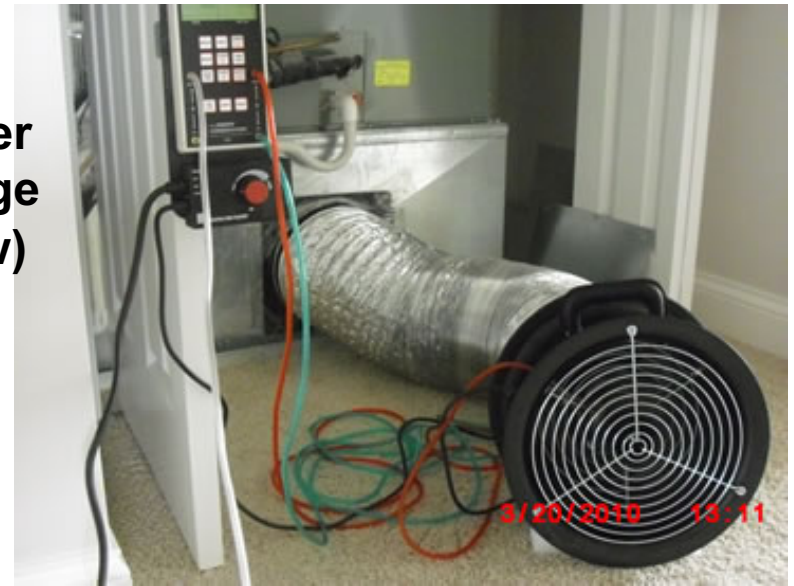
TrueFlow (HVAC airflow rates)
