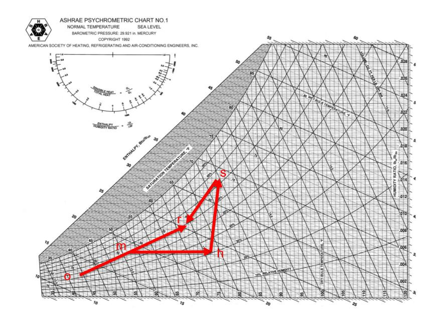
Additional Problem: Conditioned air is supplied to a space at a dry bulb of 54 °F and relative humidity of 90% at the rate of 1,500 CFM. The sensible heat ratio for the space is 0.8, and the space is to be maintained at the 75 °F.
