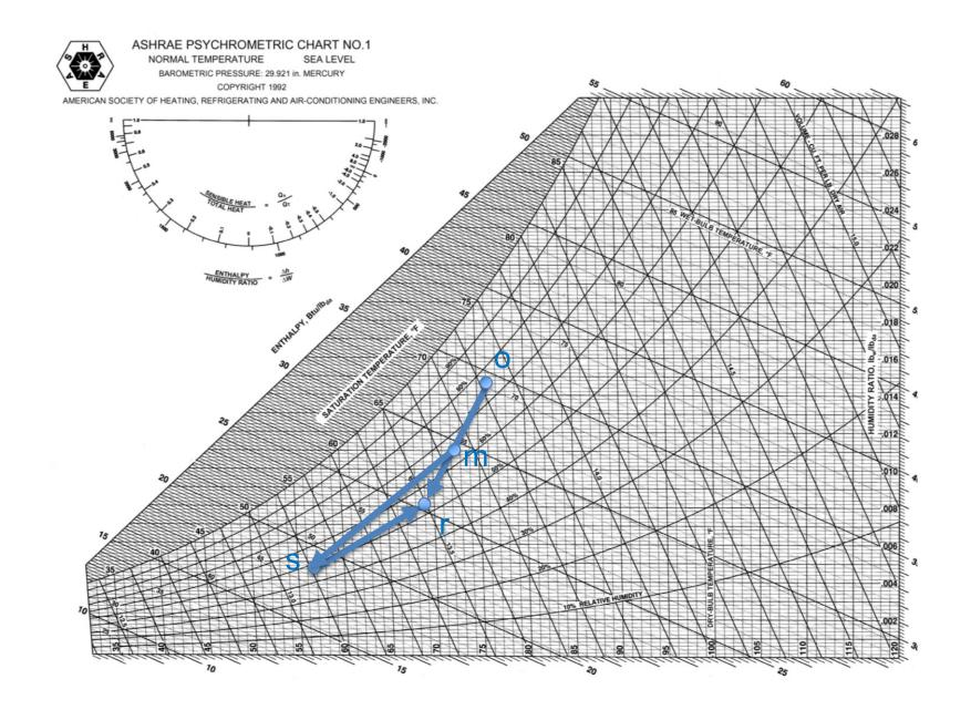
A typical AC system with the influence of the fan falls this process
