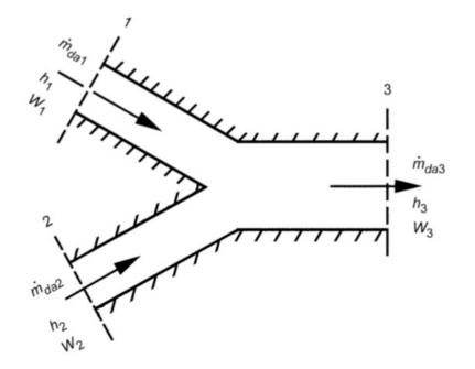
$$\dot{m}_{da1}h_1 + \dot{m}_{da2}h_2 = \dot{m}_{da3}h_3$$
