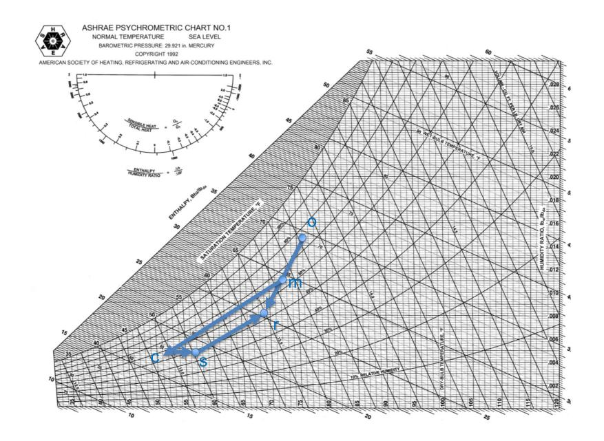
A typical winter heat conditioning space heat loss follows the following schematics
