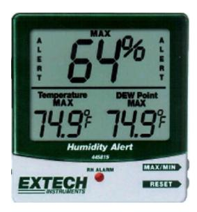
$$\phi = \left[\frac{x_{w}}{x_{ws}}\right]_{T,P} = \frac{p_{w}}{p_{ws}}$$
