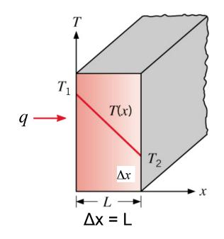
Here  $T_1$  and  $T_2$  are the surface temperatures at  $x_1$  and  $x_2$ Notice that this equation differs from the last by a minus sign I suggest you use the  $\Delta T/\Delta x$  formulation and note that heat will always flow from high to low temperature
