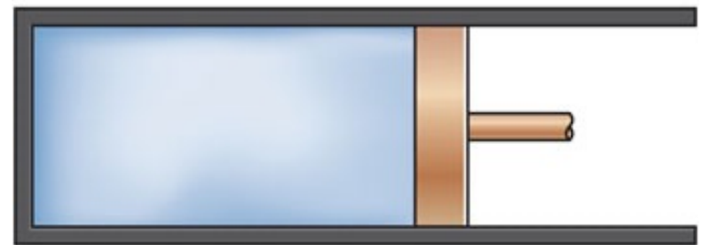
(b) Quasi-equilibrium expansion and compression of a gas
