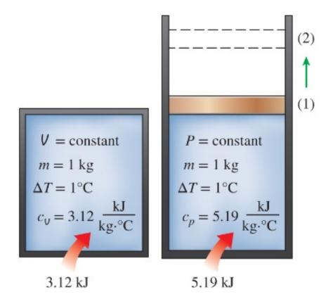
Let's start from the fixed mass in a stationary closed system that undergoes a constant volume process
