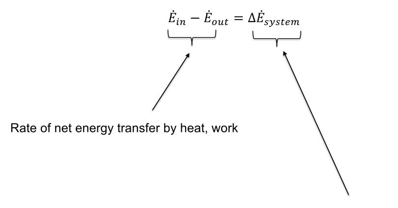
Rate of change in internal, kinetic, potential, ..., energies
