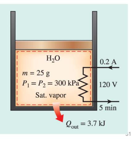
$$W_b = P_0(V_2 - V_1)$$
