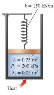
$$V_2 = 2V_1 = 2(0.05 m^3) = 0.1 m^3$$
