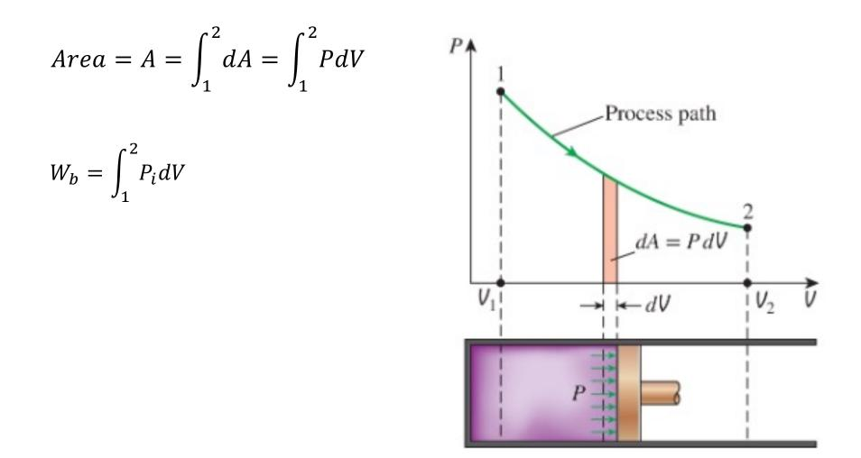
The net work done during a cycle is the difference between the work done by the system and the work done on the system:
