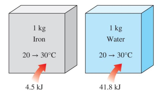
• Specific heat is defined as the energy required to raise temperature of a unit mass of substance by one degree
