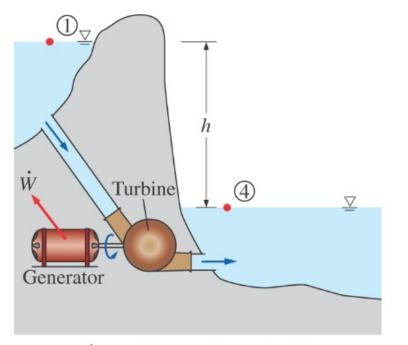
$\dot{W}_{\text{max}} = \dot{m}\Delta e_{\text{mech}} = \dot{m}g(z_1 - z_4) = \dot{m}gh$ since  $P_1 \approx P_4 = P_{\text{atm}}$  and  $V_1 = V_4 \approx 0$
