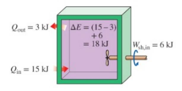
The net change (increase or decrease) in the total energy of the system during a process is equal to the difference between the total energy entering and the total energy leaving the system during the process
