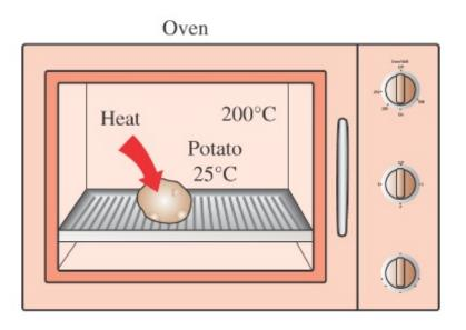
A well-insulated electric oven is being heated through its heating element. If the entire oven, including the heating element is taken to be the system, determine whether there is a heat or work interaction.
