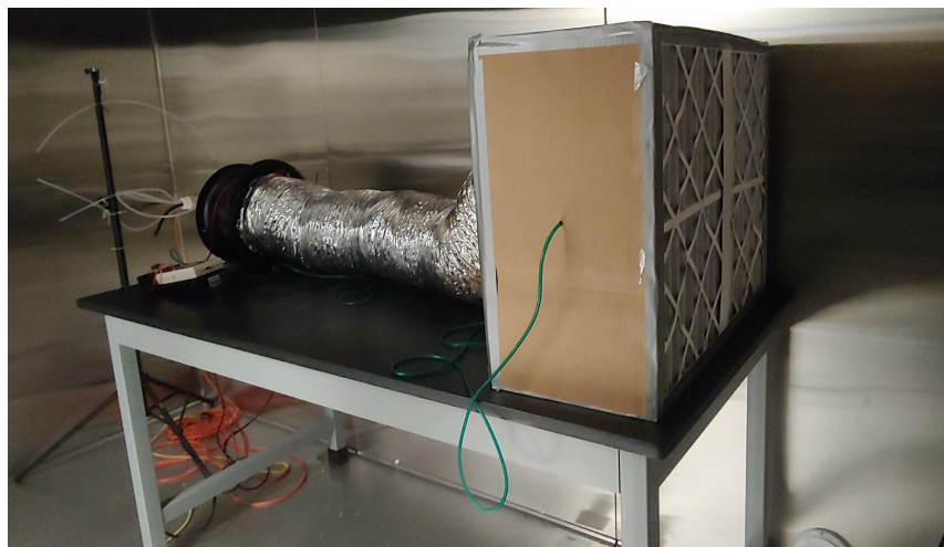
168 169 Figure S2. Chamber test setup for measuring VOC removal efficiency of a new 10 cm (4 inch) depth 170 carbon-impregnated MERV 13 filter at Portland State University.
