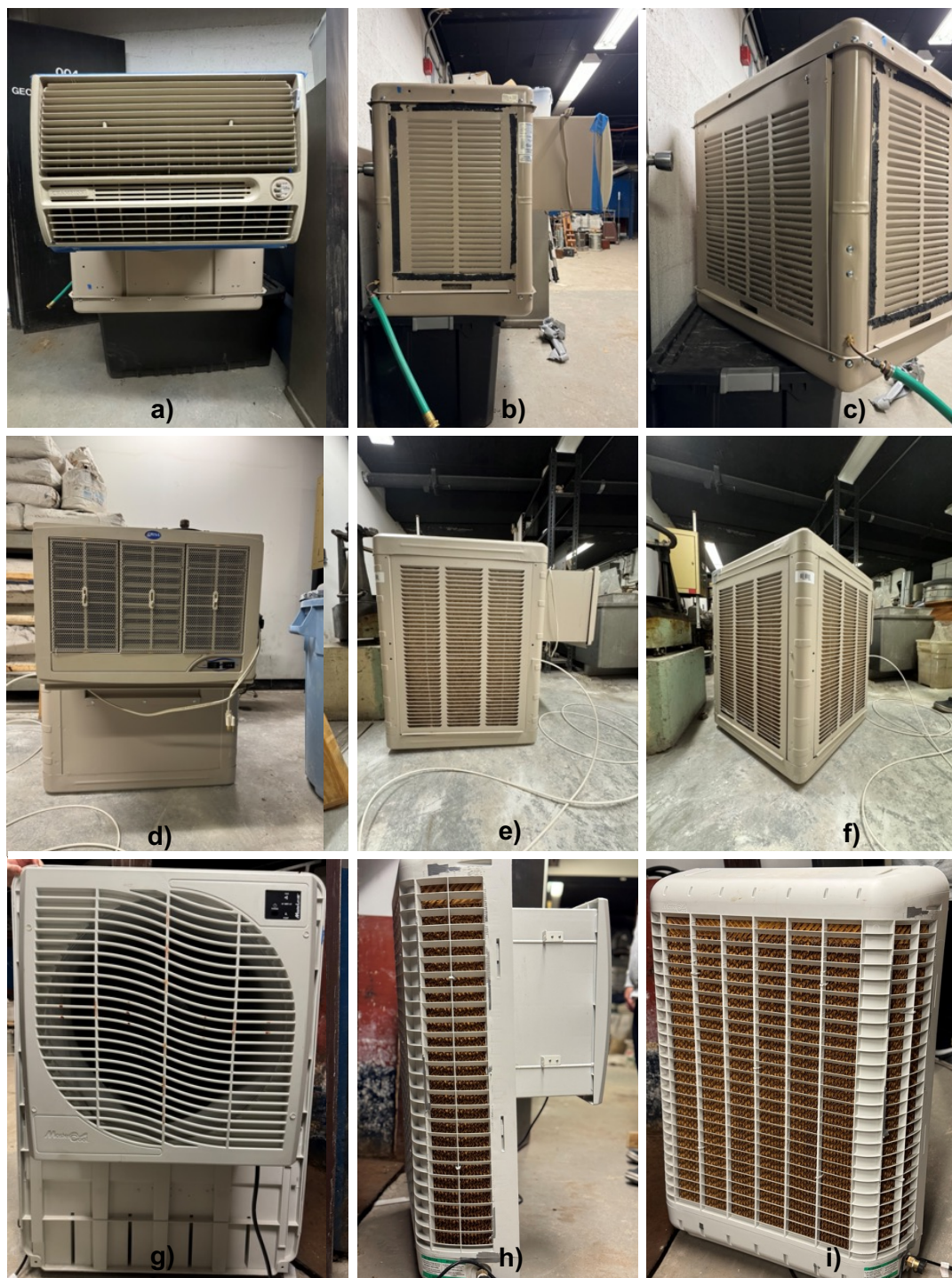
Figure S1. Three horizontal-flow (through-the-window/wall) residential ECs acquired for laboratory testing: a-c) Essick RN35W, d-f) Phoenix/Brisa BW4002, and g-i) MasterCool MCP44.
