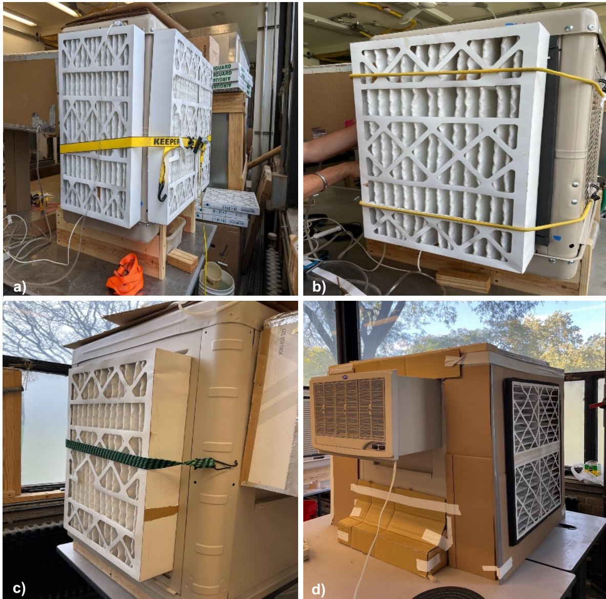
322 323 Figure 2. Filter and filter media attachment methods tested in the laboratory: (a) tie-down ratchet straps, 324 (b) bungee cords, (c) bungee straps, and (d) custom plenum-like intake and housing for filters.
