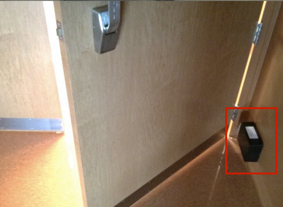
Differential Pressure Sensors (in black box with batteries, attached with adhesive), data logger, clear tube running to outer door frame
